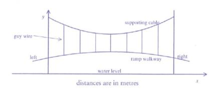
The equation of the ramp walkway is  $y = -0.001x^2 + 0.062x + 18.04$
